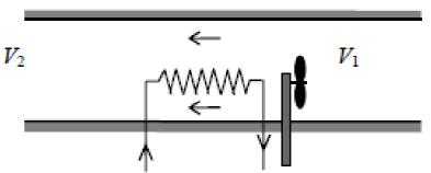
A smoking lounge is to accommodate 15 heavy smokers. The minimum fresh air requirement for smoking lounges is specified to be 30 L/s per person (ASHRAE, Standard 62, 1989). Determine the minimum required flow rate of fresh air that needs to be supplied to the lounge, and the diameter of the duct if the air velocity is not to exceed 8 m/s.
