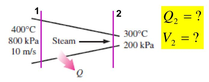
5-42 Heat is lost from the steam flowing in a nozzle. The velocity and the volume flow rate at the nozzle exit are to be determined.
